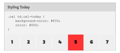
The cal-today class shows that the today class is part of the cal module. We are also increasing the specificity which will have this style override the default style. Alternative selector choices could've included just a plain td.cal-today which would have worked as long as it was declared after the default state rule. Had we used just .cal-today as our selector, we would've had to resort to using !important to get this style to work.
